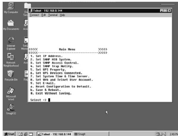
Fig.42 NetAgent Telnet window
